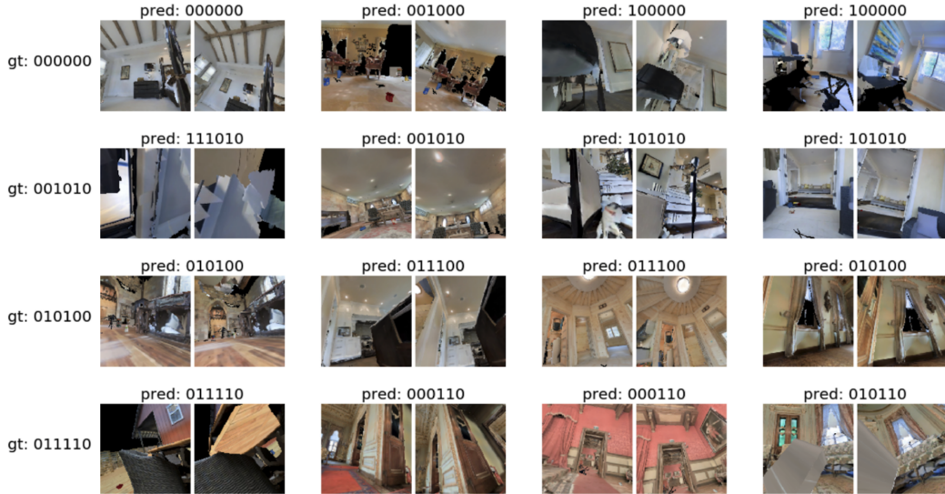
Figure 4: Relative camera pose estimation task. 010100 means relative x translation is -0.3\text{m} , relative y translation is 0.3\text{m} , relative z translation is -0.3\text{m} , yaw is +15^\circ , pitch is -15^\circ and roll is -15^\circ . Each row corresponds to a specific relative camera pose and contains 4 pairs of RGB images.
